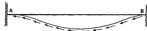
Fig. 13. Clamped-clamped beam subjected to uniformly distributed follower forces: one of the simplest example of pseudo-divergence system
