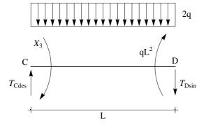
$$-T_{\text{Cdes}} + T_{\text{Dsin}} + 2 q L = 0 (27)$$
